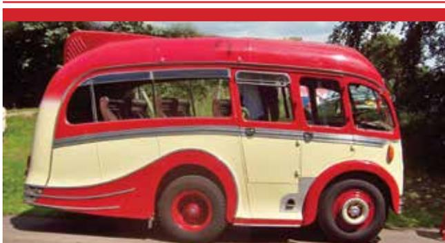
Special buses commissioned for Guernsey still feature full sized wheels to minimise passenger discomfort when mounting pavements
